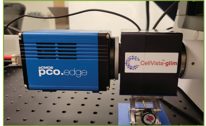
Figure 1 – GLIM setup using the X-Cite NOVEM (left, green box) and PCO camera (right, blue box). The Phi Optics GLIM module is the black box in the right image between the PCO camera and the microscope.
